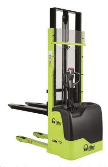
This compact, powerful and robust stacker is the ideal solution for working in confined spaces. The reduced width (800 mm), the lateral driving system and the wide mast positioning allow great manoeuvrability, stability and visibility. Built-in battery charger with integrated cable and plug make it a plug and play unit!
